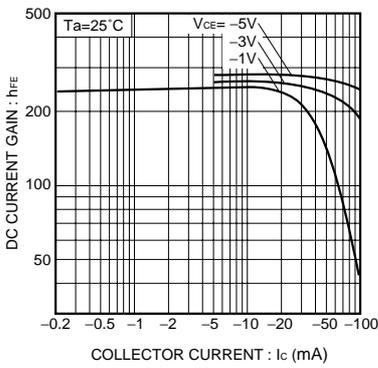
Fig.4 DC current gain vs. collector current (I)
