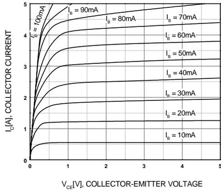
Figure 1. Static Characteristic
