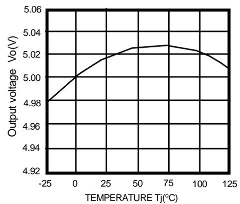
Figure 4. Output Voltage vs. Temperature( $T_j$ )
