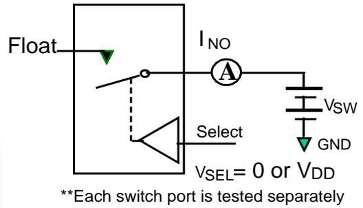
**Figure 5. Off Leakage**
