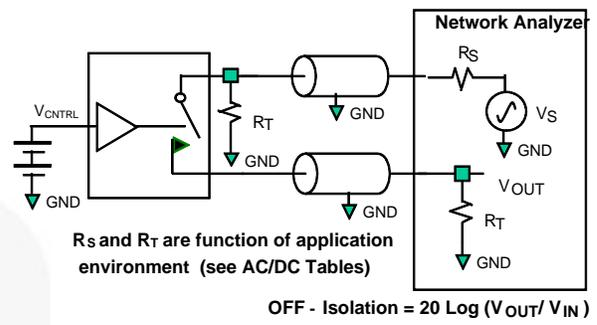
OFF - Isolation =  $20 \text{ Log } (V_{OUT} / V_{IN})$
