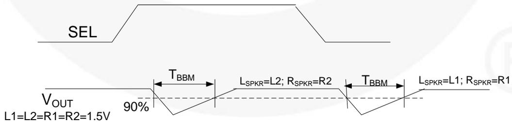
**Figure 9. Break Before Make Interval Timing**
