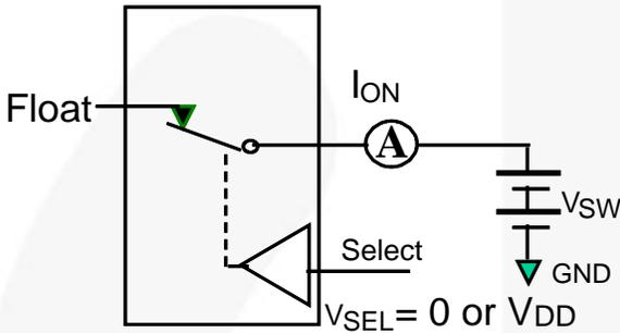
**Figure 6. On Leakage**
