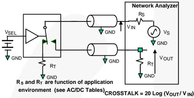
CROSSTALK =  $20 \text{ Log } (V_{OUT} / V_{IN})$
