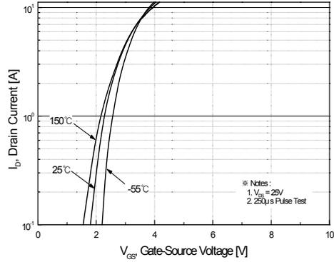
**Figure 2. Transfer Characteristics**
