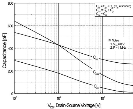
**Figure 5. Capacitance Characteristics**
