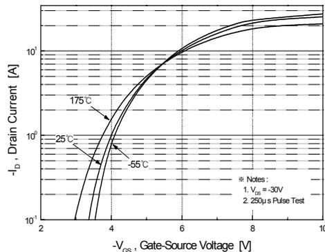
**Figure 2. Transfer Characteristics**
