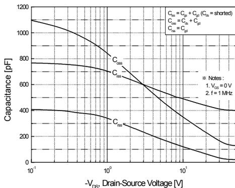
**Figure 5. Capacitance Characteristics**
