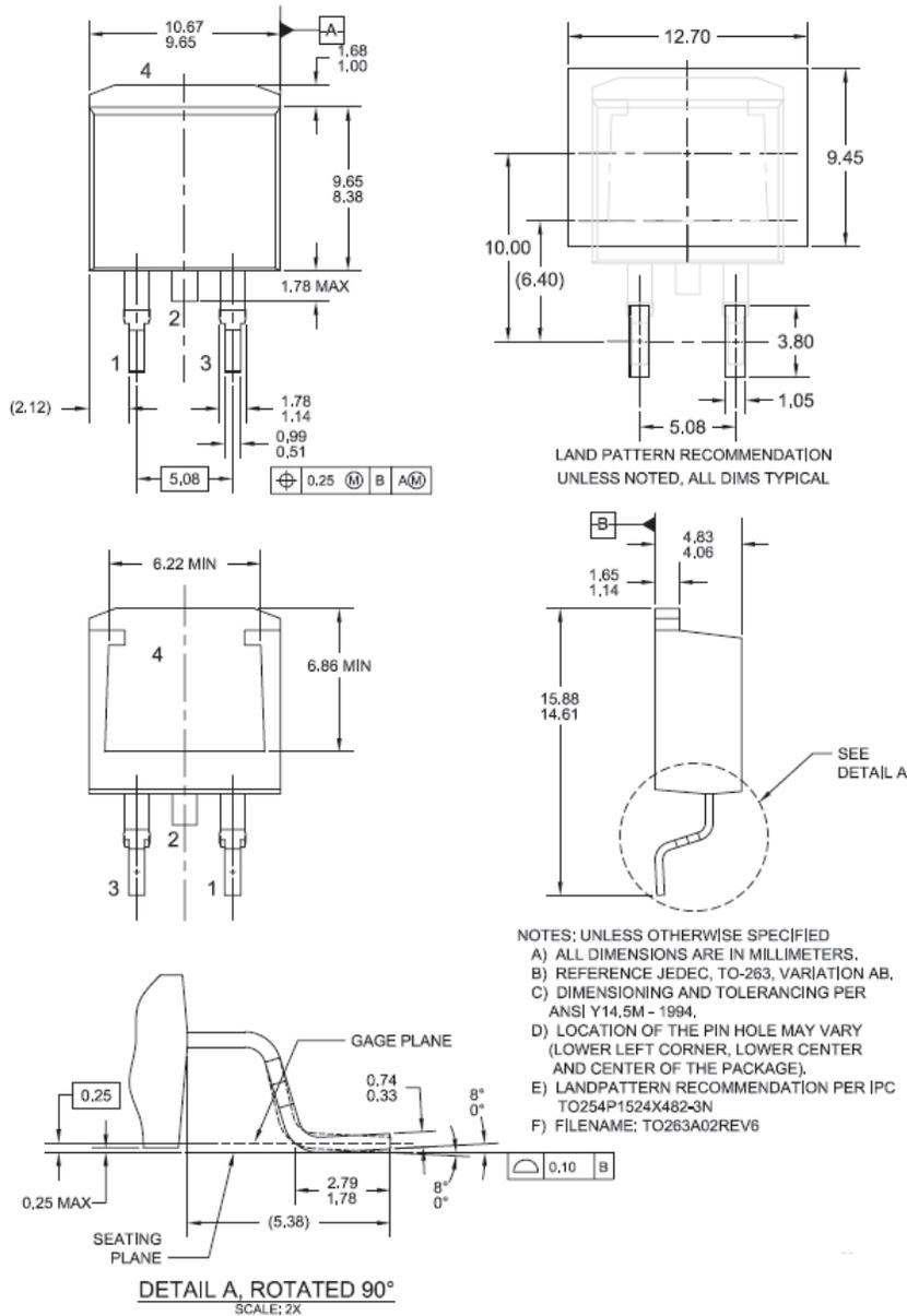
**Figure 16. TO263 (D<sup>2</sup>PAK), Molded, 2-Lead, Surface Mount**
