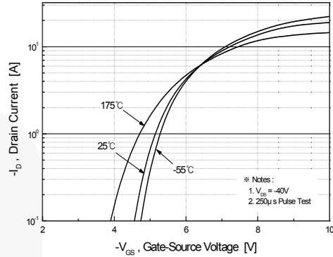
**Figure 2. Transfer Characteristics**
