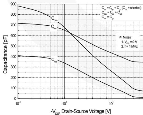
**Figure 5. Capacitance Characteristics**
