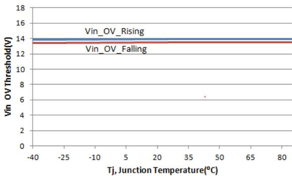
**Figure 21. V<sub>BUS\_VOVL0</sub> vs. Temperature**
