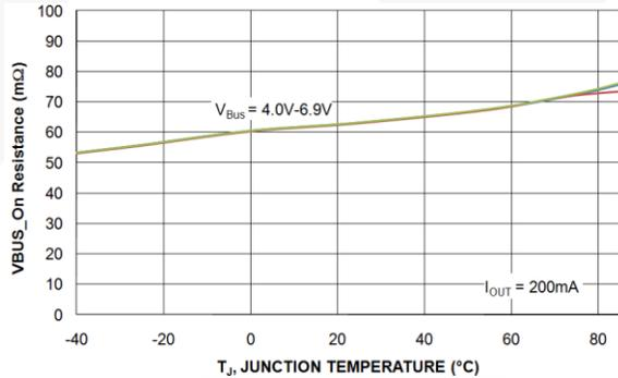
Figure 12.  $V_{BUS}$  On Resistance ( $m\Omega$ ) vs. Temperature
