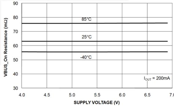
Figure 14.  $V_{BUS}$  On Resistance ( $m\Omega$ ) vs. Supply Voltage
