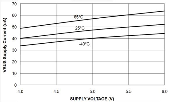
Figure 10.  $V_{BUS}$  Quiescent Current vs. Supply Voltage
