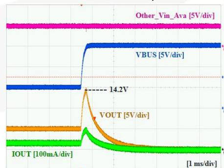
**Figure 30.  $V_{BUS}$  Over-Voltage Protection Response ( $V_{BUS}=5$  V  $\rightarrow$  15 V,  $V_{IN}=5$  V,  $EN=HIGH$ ,  $V_{IN\_SEL}=LOW$ ,  $C_{OUT}=4.7$   $\mu F$ ,  $R_L=150$   $\Omega$ )**
