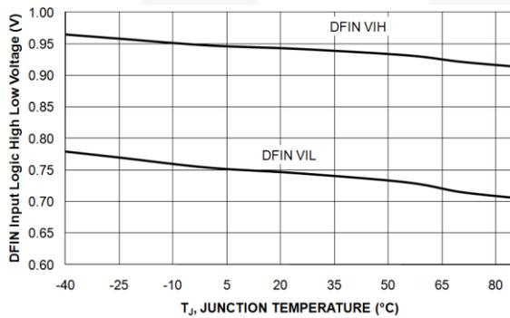
**Figure 17. DF\_IN Logic HIGH & Low Voltage vs. Temperature**
