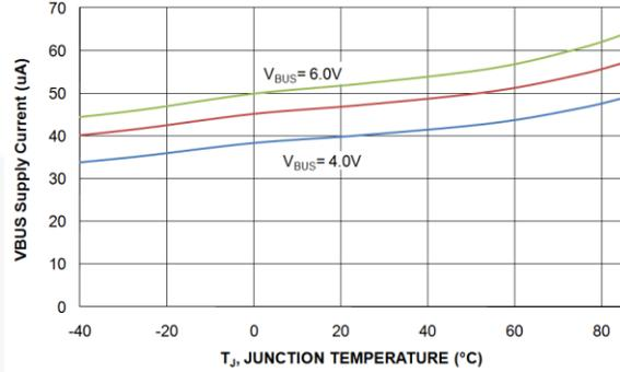
Figure 8.  $V_{BUS}$  Quiescent Current ( $I_Q$ ) vs. Temperature
