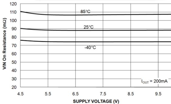
Figure 13.  $V_{IN}$  On Resistance ( $m\Omega$ ) vs. Supply Voltage
