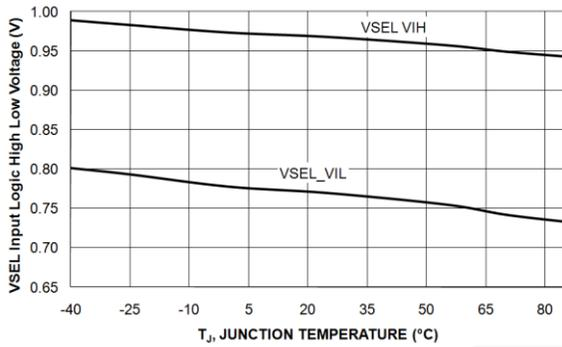
**Figure 15. V<sub>IN\_SEL</sub> Input Logic HIGH & Low Voltage vs. Temperature**
