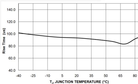
**Figure 22. V<sub>OUT</sub> t<sub>R</sub> vs. Temperature**
