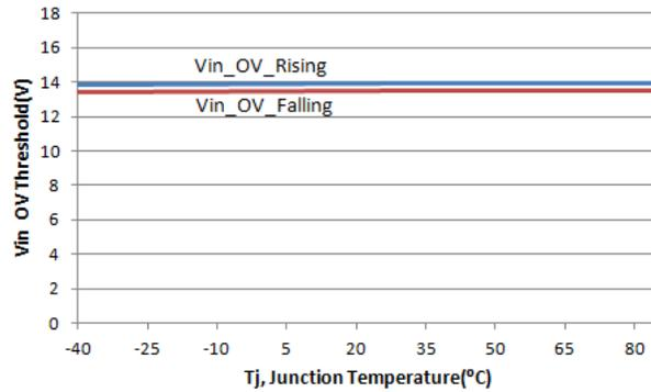
**Figure 20. V<sub>IN\_VOVL0</sub> vs. Temperature**
