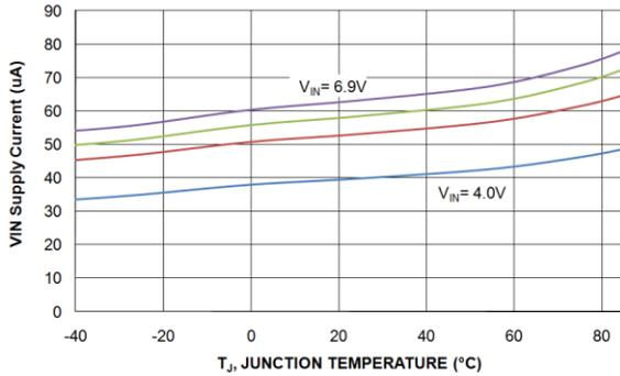
Figure 7.  $V_{IN}$  Quiescent Current ( $I_Q$ ) vs. Temperature
