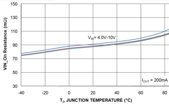
Figure 11.  $V_{IN}$  On Resistance ( $m\Omega$ ) vs. Temperature
