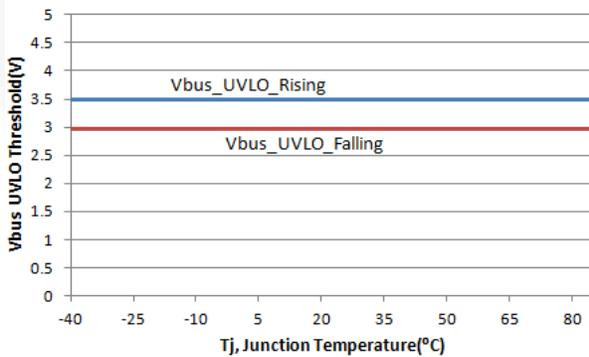
**Figure 19. V<sub>BUS\_VULVO</sub> vs. Temperature**
