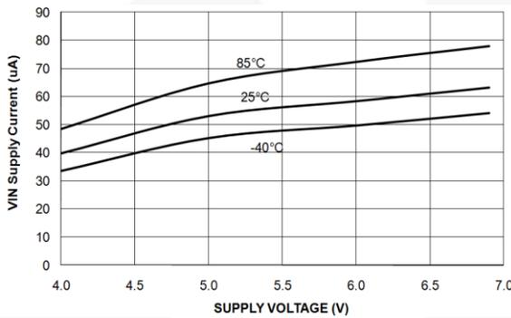
Figure 9.  $V_{IN}$  Quiescent Current vs. Supply Voltage
