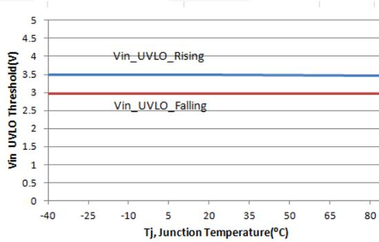
**Figure 18. V<sub>IN\_VULVO</sub> vs. Temperature**
