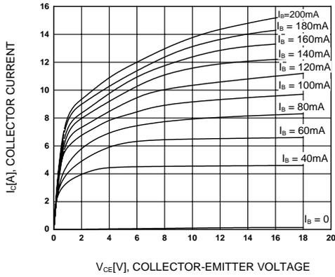
Figure 1. Static Characteristic
