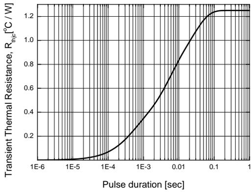
Figure 7. Thermal Resistance
