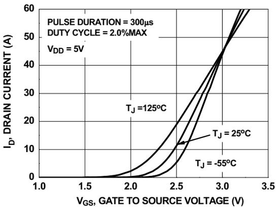
Figure 5. Transfer Characteristics
