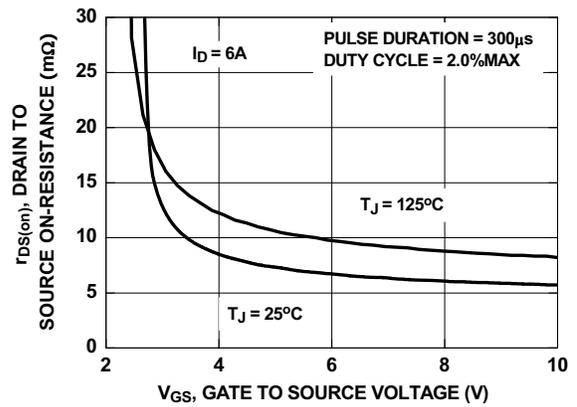
Figure 4. On-Resistance vs Gate to Source Voltage
