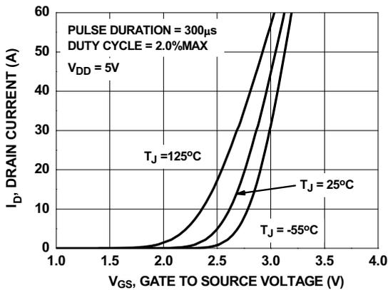
Figure 16. Transfer Characteristics
