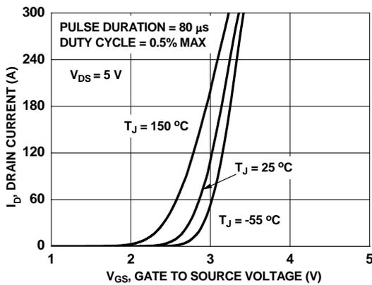
Figure 5. Transfer Characteristics
