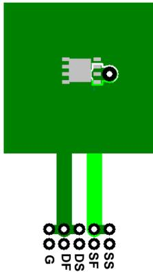
a. 38  $^{\circ}\text{C}/\text{W}$  when mounted on a 1 in<sup>2</sup> pad of 2 oz copper
