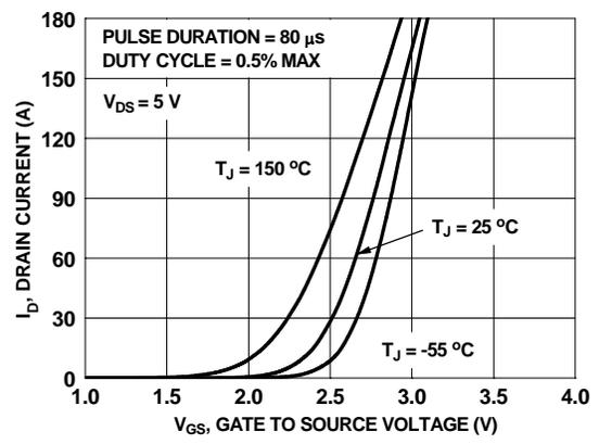
Figure 5. Transfer Characteristics
