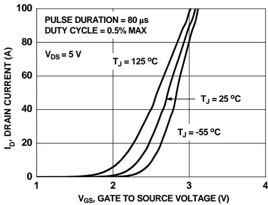
**Figure 5. Transfer Characteristics**
