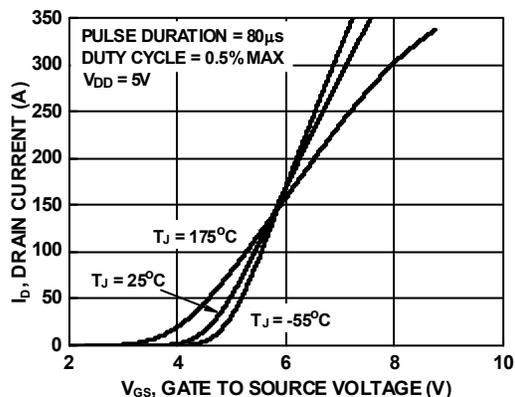
Figure 7. Transfer Characteristics
