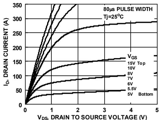
Figure 9. Saturation Characteristics
