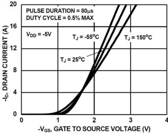
Figure 7. Transfer Characteristics
