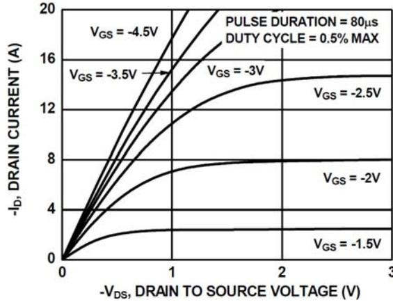
Figure 8. Saturation Characteristics
