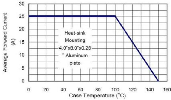
Figure 1. Maximum Derating Curve for Output Current
