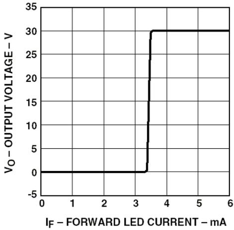
Figure 13. Transfer characteristics.
