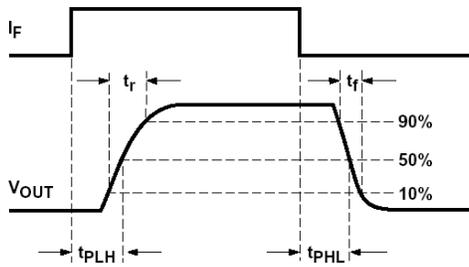
Figure 15. Propagation Delay Test Circuit and Waveforms.
